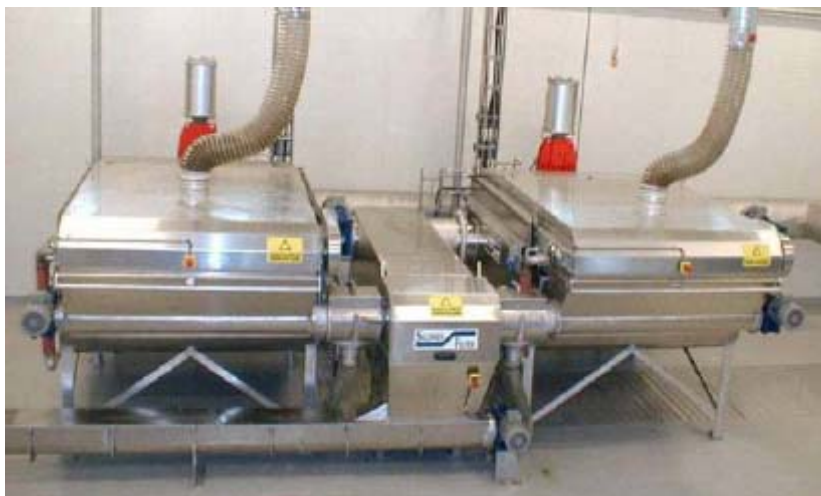
Figure 5-2 Parallel Salsnes Filters
